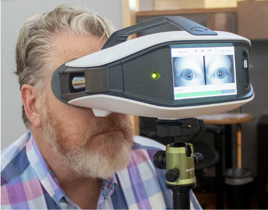
EyeStat delivers five light puffs of food-grade carbon dioxide at random intervals to the corner of the eyes over a 20-second time frame to assess the blink reflex.
