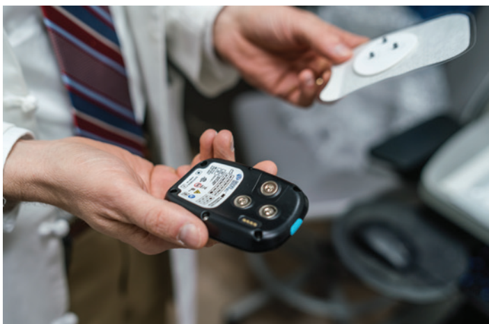
Jonathan Halford, M.D. , worked with device company Brain Sentinel, Inc. , to develop the first FDA-approved system to detect generalized tonic-clonic seizures using a wearable device that continuously records EMG activity in the bicep.
